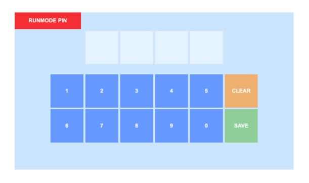
You can set the four digits passcode by pressing the keypads. There is <u>no</u> <u>backspace key</u>: you have to clear <u>all</u> digits in case you made a typing error by pressing CLEAR. Once you have decided about your passcode press the SAVE button.
