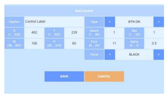
Same as for editing a control, press **SAVE** to record your changes (You can also change the control type) or **CANCEL** to return to the previous screen. You can use X, Y, W and H parameters to properly align your controls.
